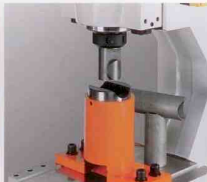
*Urethane spring stripper for minimal deformation.
