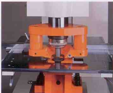
*Urethane spring stripper for minimal deformation.
